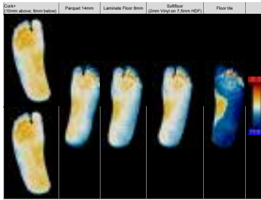
Comparative thermography images taken after 80 seconds, standing on the test surface
